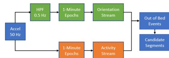
**Study Data.** Three-axis accelerometer data were acquired at 50 Hz, and processed as Orientation and Activity data streams in 1-minute epochs. These were used to detect Out-of-Bed (OOB) events. Sets of epochs between OOB events are called Segments (SEG).
