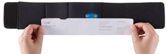
3. Remove the liner covering the electrode prior to placing the device on your leg. **Remember to keep the liner as it should be re-applied to protect the electrode when not in use.**
